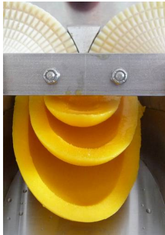
Mango being sliced by concentric cupping knife attachment.
